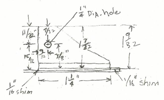
The brackets are approximately ¾" wide. The shim is necessary because of the attachment angle that is riveted to the channel. Everything else is pretty much the same as the original installation. If you do not have enough adjustment available in the rod ends on the F-659 flap link, it may be necessary to make a couple of new links that are slightly longer.
